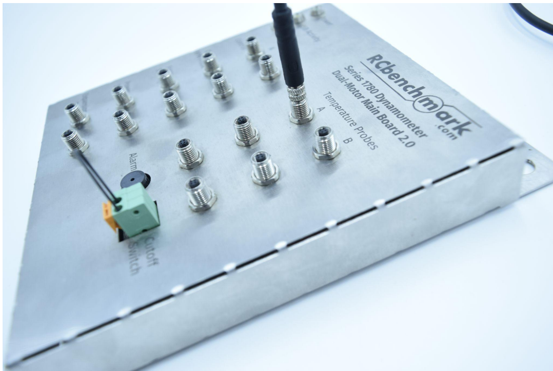
Fig. 1: Insert the temperature probe in one of the "Temperature Probes" plugs.
