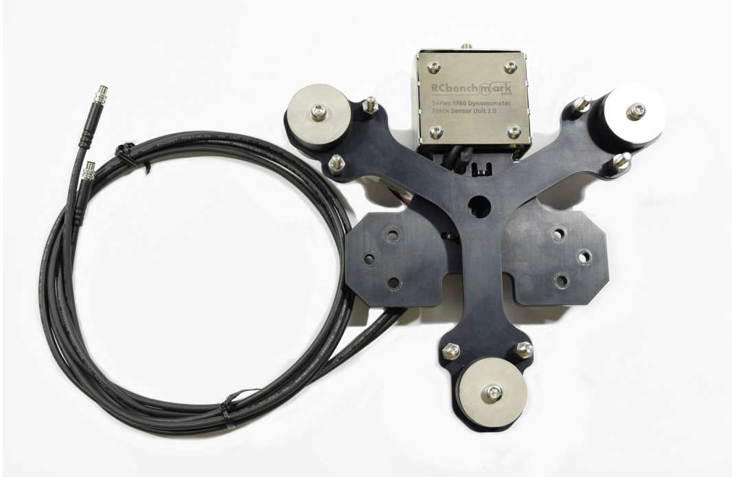
Fig 4.14: Load measurement unit assembly
