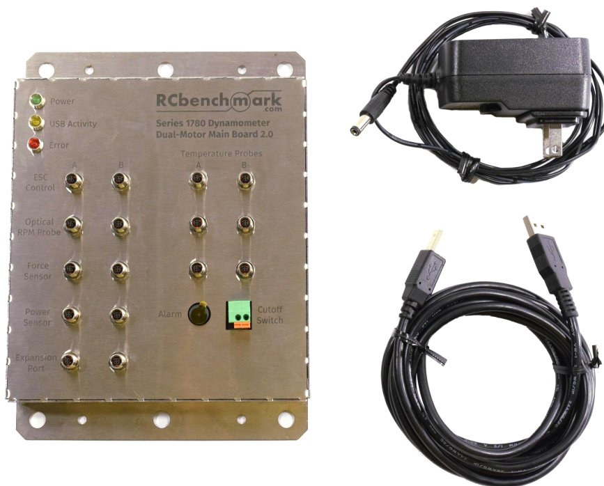
Fig. 4.34: Photo of dual main board with USB cable and power adapter
