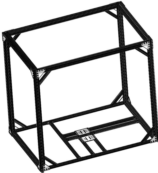
Fig. 3.32: Enclosure with 2-axis railing system inside
