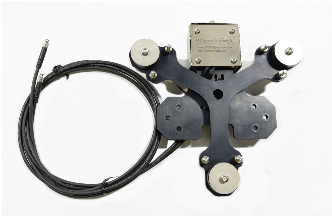
Fig 4.14: Load measurement unit assembly
