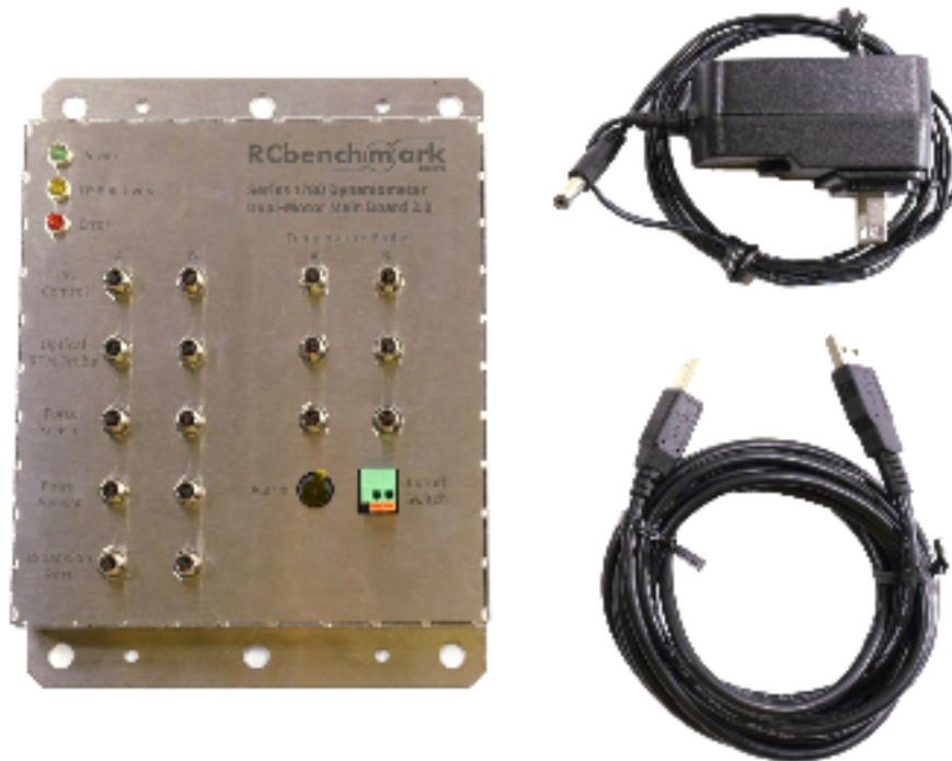
Fig. 4.33: Photo of dual main board with USB cable and power adapter
