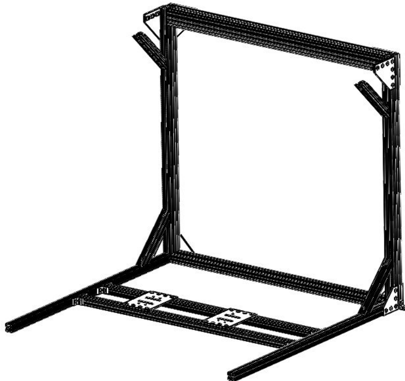
Fig. 3.28: 1-axis railing system setup on the bottom beams
