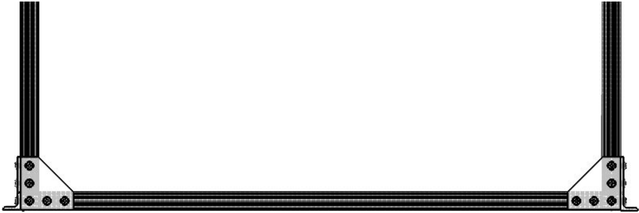
Fig. 3.22: 1-1/2" x 3" T-slotted frame with two vertical beams (can be 4' or 6' beams)
