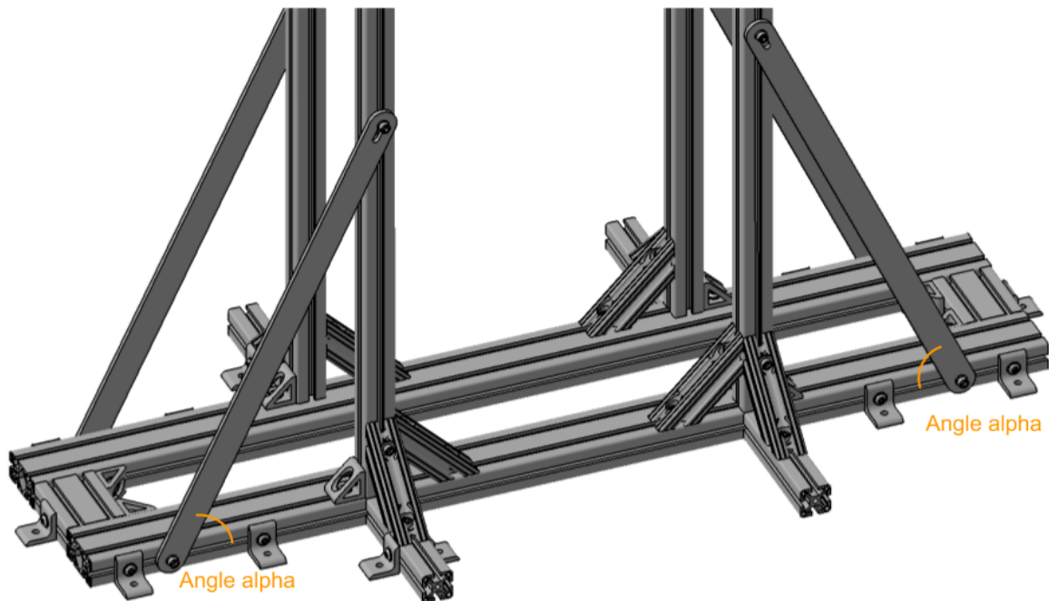
Fig. 6.2: Angle \alpha (alpha) for each stand on a face-to-face setup
