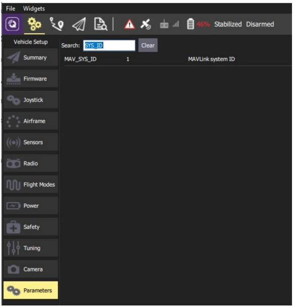
You also need to change the position forward script on each quadcopter so the flight controller receives position messages from a single quadcopter. Connect to your drone through the
