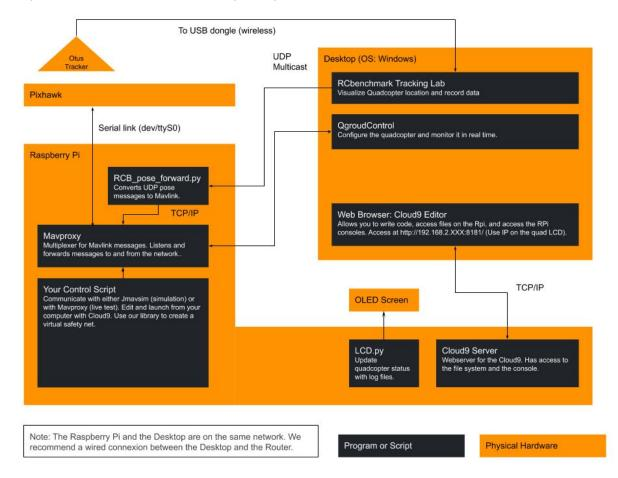
You Otus Quadcopter's brain is the flight controller, the Pixhawk. It controls the motors and does all the sensor processing for the flight. The flight controller communicates with the outside using a protocol named Mavlink. The ground control software and your control script, for example, communicate with the Pixhawk using Mavlink packets. Here is a summary of the functions performed by the **flight controller**:
